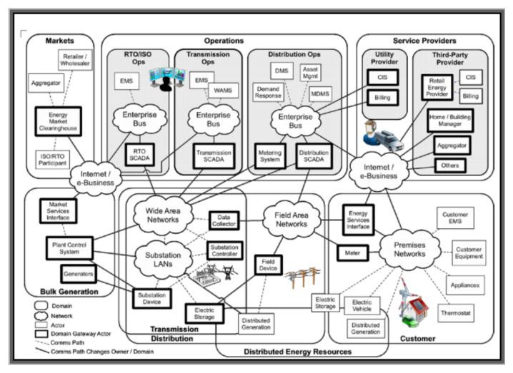
Figure 2: Conceptual Reference Diagram for Smart Grid Information Networks Error! Bookmark not defined.
